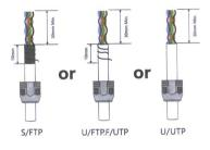
Pan out all four twisted pairs, following the color coding label and allocate each conductors into proper slots on wiring cap.
