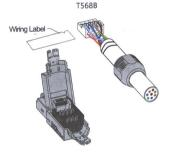
Place the wiring cap onto plug, use plier to clamp wiring cap until it completely snap-in to effect the connection.
